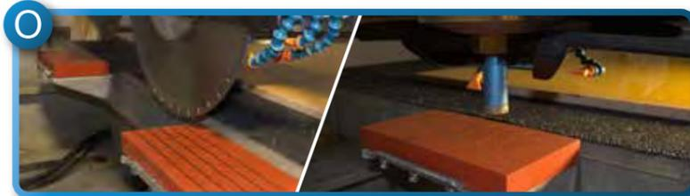
**Redressing Devices for Disc and Core Drill including Automatic Management Software**
