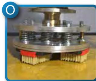
**Spring-Loaded Head for Surfaces Honing and Leathering**
